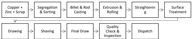
Rods, wires and tubes of copper / brass are made out of scraps, cathode and ingots of copper and zinc. Scrap is first segregated and then graded as per the alloying requirements of the customers. These segregated lots are sent for melting and casting to billets on job work. Thereafter, rods, wires and tubes are extruded from billets for further processes of drawing, surface treatment and annealing.
